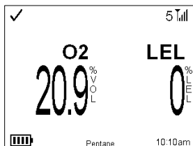
Home screen - two installed sensors
