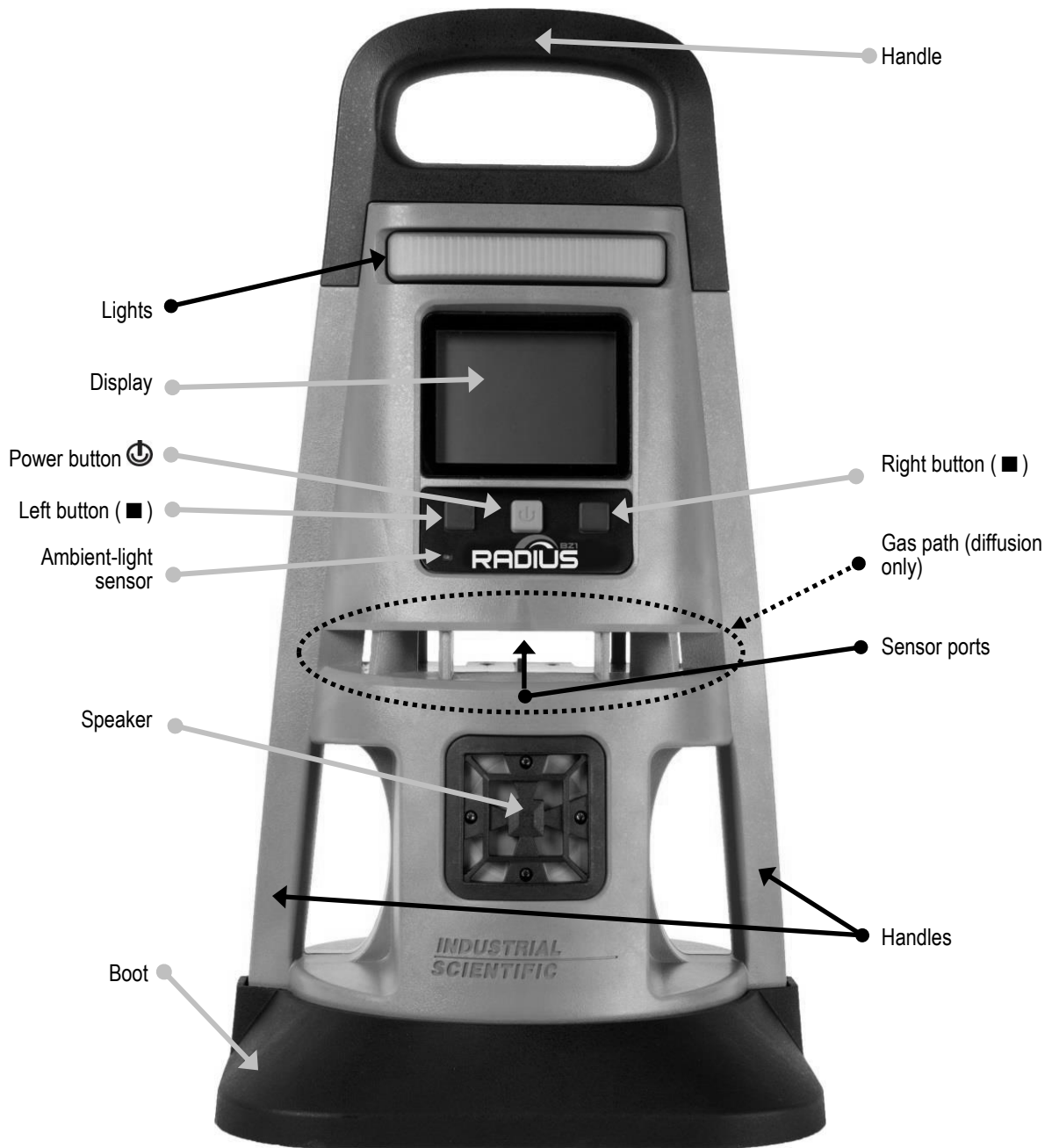
Figure 3.1.A Hardware overview Radius BZ1 (front view; diffusion)
