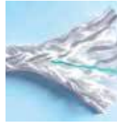
Coated core rope, double plaited.
