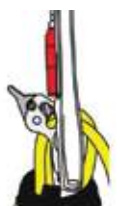
Cam Disengaged For lowering
