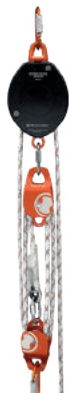
GORDON PULLEY SYSTEM 1:5 A-120-3+ L-0741-Length (R-064) Semi-static rope 10.5 mm Sewn eyelets rope length corresponds to lifting height times 5
