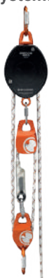
GORDON PULLEY SYSTEM 1:3 A-120-3+ L-0741-Length (R-064) Semi-static rope 10.5 mm Sewn eyelets rope length corresponds to lifting height times 3
