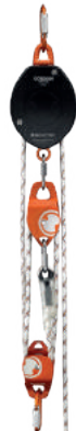
GORDON PULLEY SYSTEM 1:4 A-120-3+ L-0741-Length (R-064) Semi-static rope 10.5 mm Sewn eyelets rope length corresponds to lifting height times 4
