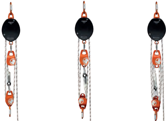
GORDON PULLEY SYSTEM 1:3 A-120-3+ L-0741-Length (R-064) Semi-static rope 10.5 mm Sewn eyelets rope length corresponds to lifting height times 3 GORDON PULLEY SYSTEM 1:4 A-120-3+ L-0741-Length (R-064) Semi-static rope 10.5 mm Sewn eyelets rope length corresponds to lifting height times 4 GORDON PULLEY SYSTEM 1:5 A-120-3+ L-0741-Length (R-064) Semi-static rope 10.5 mm Sewn eyelets rope length corresponds to lifting height times 5
